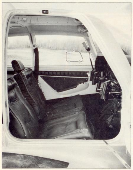
Seat design coupled with built-in arm rests makes the Mooney cabin snug but comfortable for long-duration flights. Door seal is good; air noise low.
